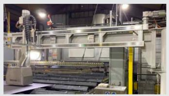
▶ Servo controlled movements to avoid contact with coated surface.
